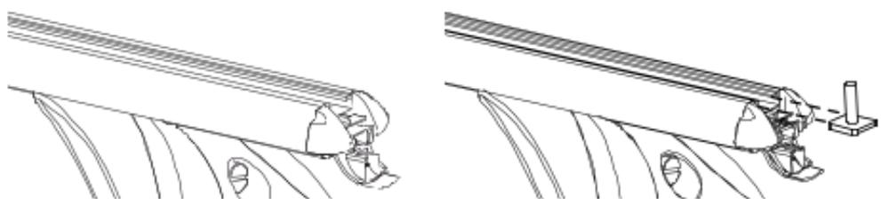
End cap can be opened to remove the rubber strip & insert T-Bolts for ease of adding accessories. You will need to cut the rubber strip to reinsert around the T-Bolts, and maintain the weatherproofing of the roof bars.
